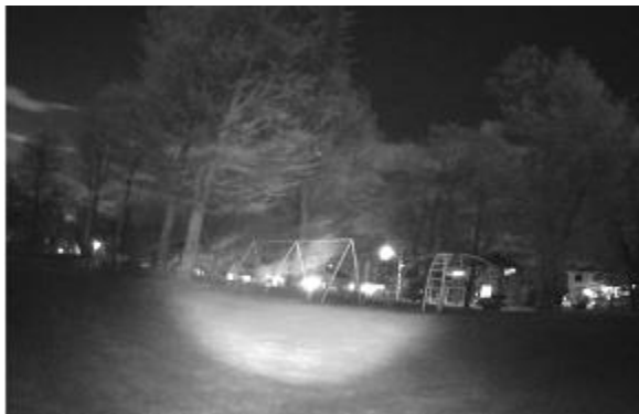
3MP camera with built-in IR Uneven illumination / center hotspot
